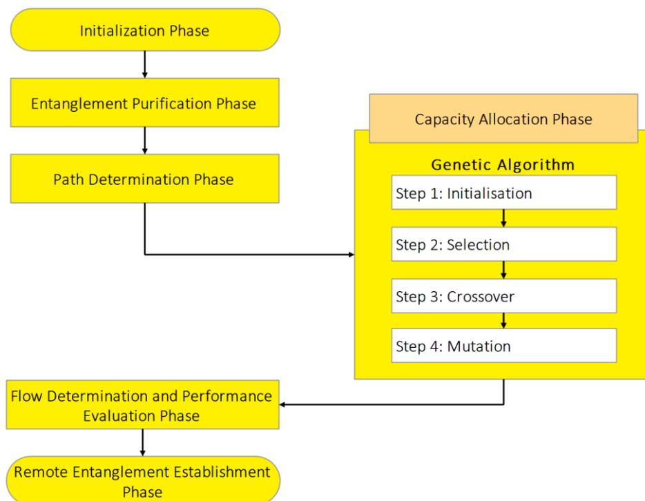
**Fig. 1.** Summary of the routing scheme: Capacity allocation scheduling scheme based on a genetic algorithm
