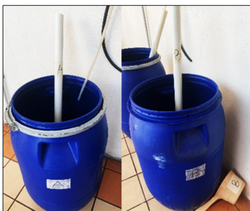
Fig. 1. Parts A and B were diluted with water in different 100 L containers
