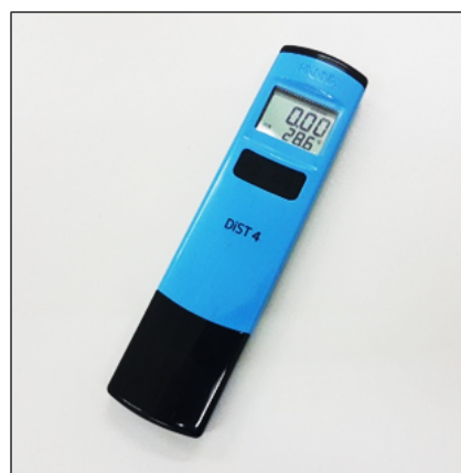
Fig. 2. EC meter (HANA instrument) for measuring the EC level of AB mix nutrients
