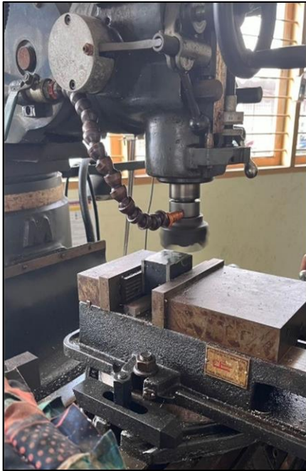
Fig. 4. Milling process to flatten magnet surface
