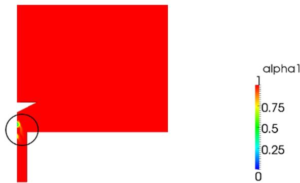
Fig. 10. Air-bubble occurrence with  $D_{cone} = 2d$
