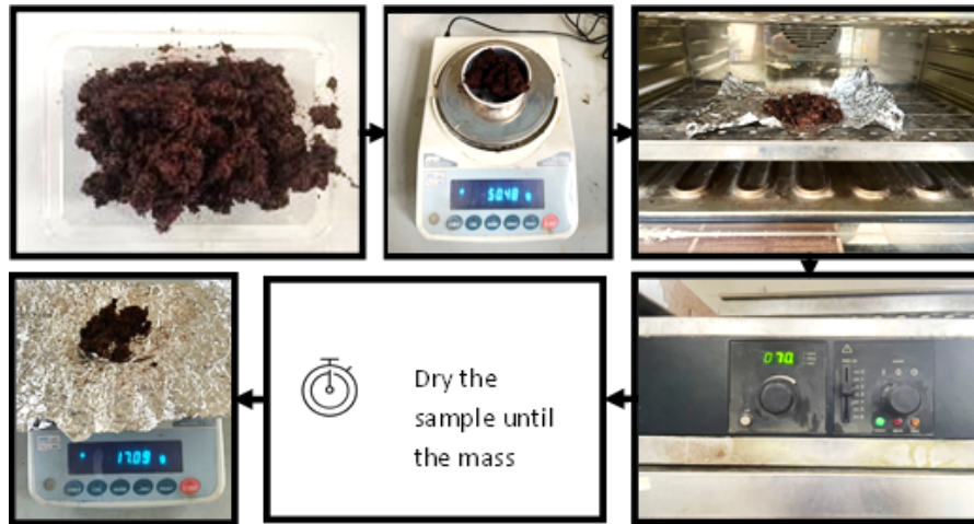
Fig. 2. The moisture content measurement process of the peat soil sample
