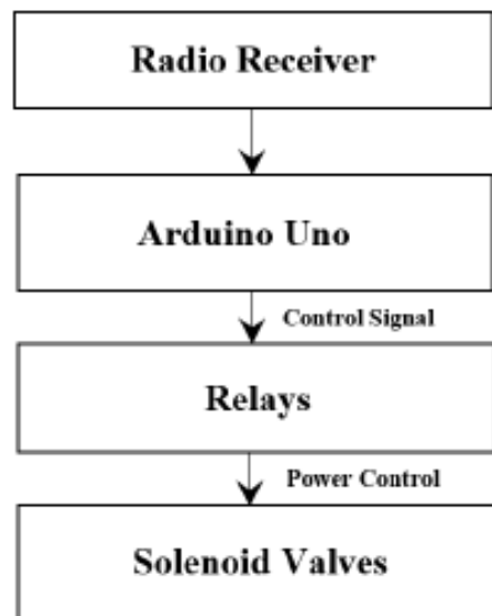
Fig. 2. Flowchart of control valves system
