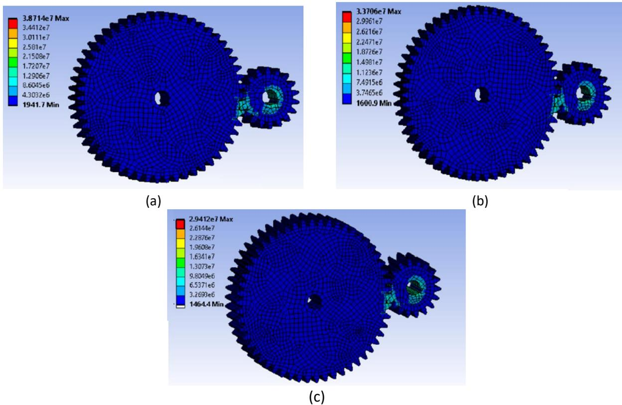
**Fig. 5.** Bending stress distribution of Kenaf-Epoxy composite gear with face width,  $b$  as (a) 30 mm (b) 35 mm and (c) 40 mm
