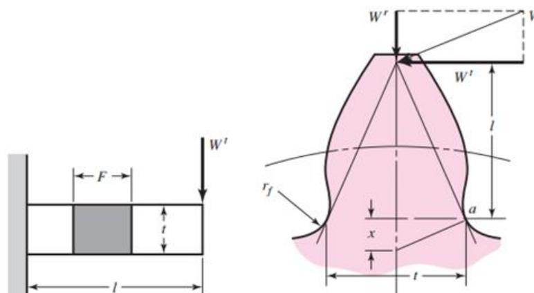
Fig. 1. A gear tooth treated as a cantilever [1]
