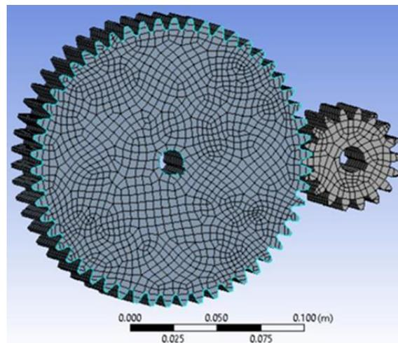
**Fig. 3.** The meshing of the gears
