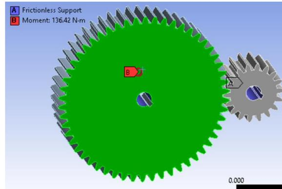
Fig. 4. The loading and boundary condition
