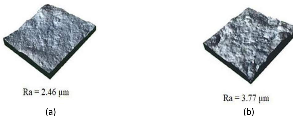
Fig. 4. 3D topographical images and average roughness results of (a) EP resin and (b) zinc oxide nano superhydrophobic coating samples
