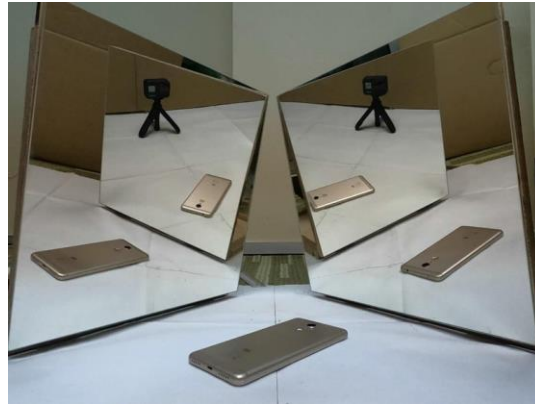
Fig. 9. Cell phone C (Mirror inclination = 80^\circ , Angle between mirror = 70^\circ )
