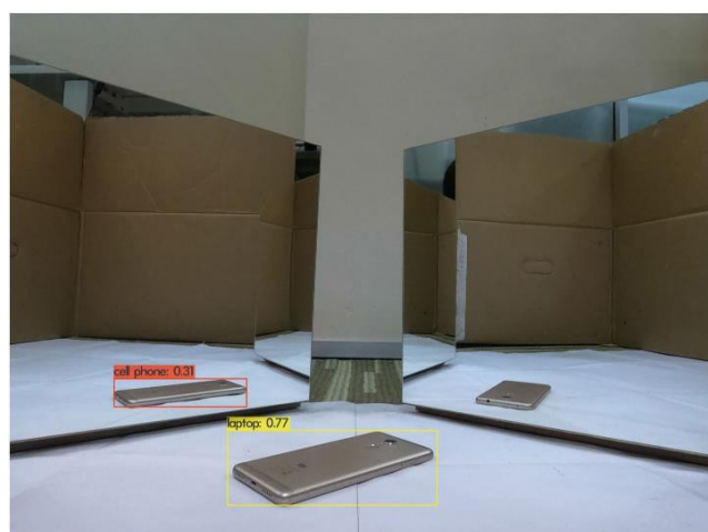
Fig. 13. Cell phone C using confidence score using YOLOv4 (Mirror inclination = 90°, Angle between mirror = 100°)
