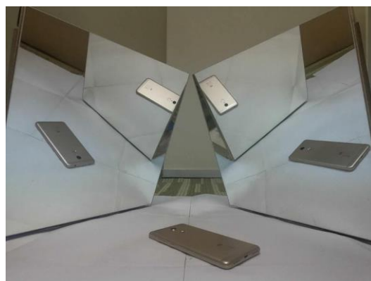
Fig. 8. Cell phone C (Mirror inclination = 70^\circ , Angle between mirror = 70^\circ )
