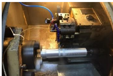
Fig. 1. Machining under MQL condition
