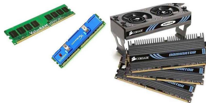
Fig. 12. Few types of DIMM with its own cooling solution
