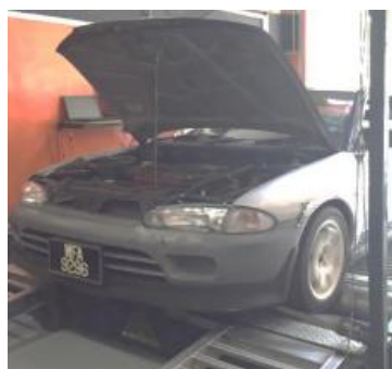
Fig. 1. Dyno test at various speeds from 1500 - 4500 rpm
