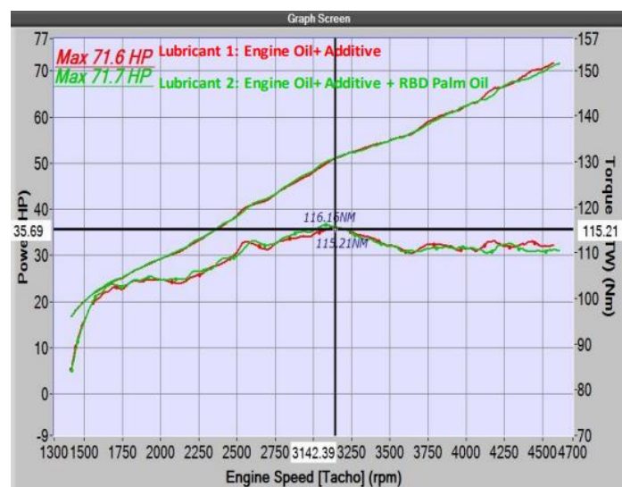
Fig. 3. Comparison of power and torque performance between engine oil + additive and engine oil + additive + RBD palm oil
