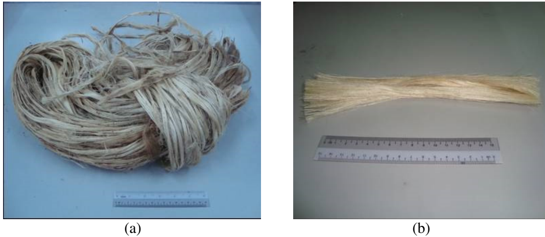
Figure 1(a) and (b): Raw materials of Kenaf bast fibres and unidirectional Kenaf bast fibres after combing, respectively
