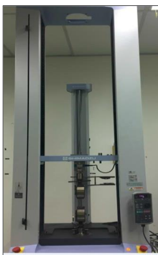
Fig. 3. Universal testing machine used during experiment
