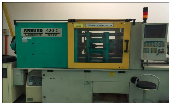
Fig. 2. Injection molding machine used in the experiment
