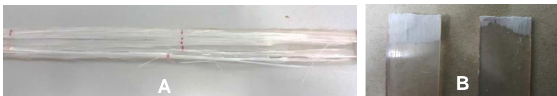
Fig. 2. (A) Fractured test specimen from preliminary tensile test and (B) Fractured test specimen after an incision was introduced
