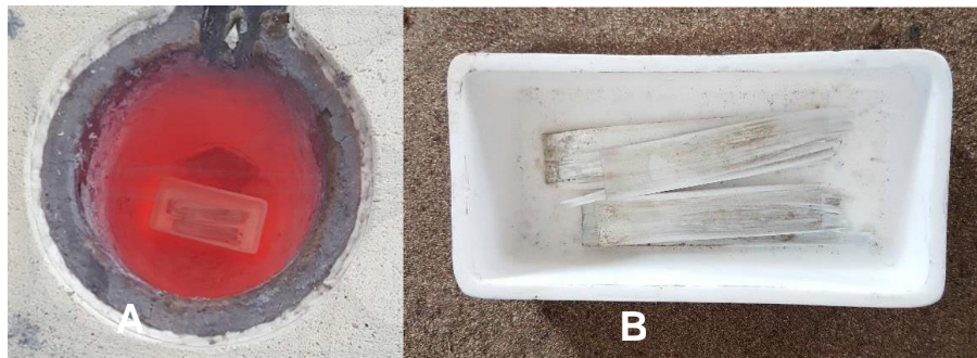
Fig. 6. (A) Specimen sample in ceramic cubicle placed in the crucible furnace and (B) Remains of fibre after burnout test
