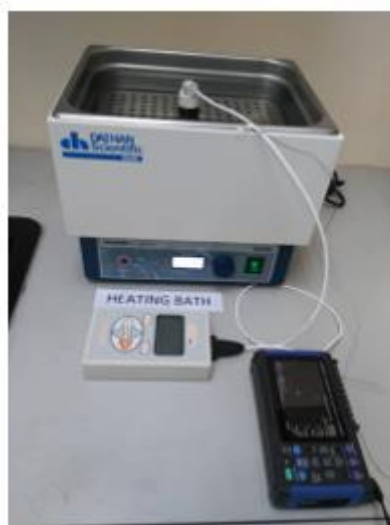
Fig. 4. Thermal conductivity experimental set-up
