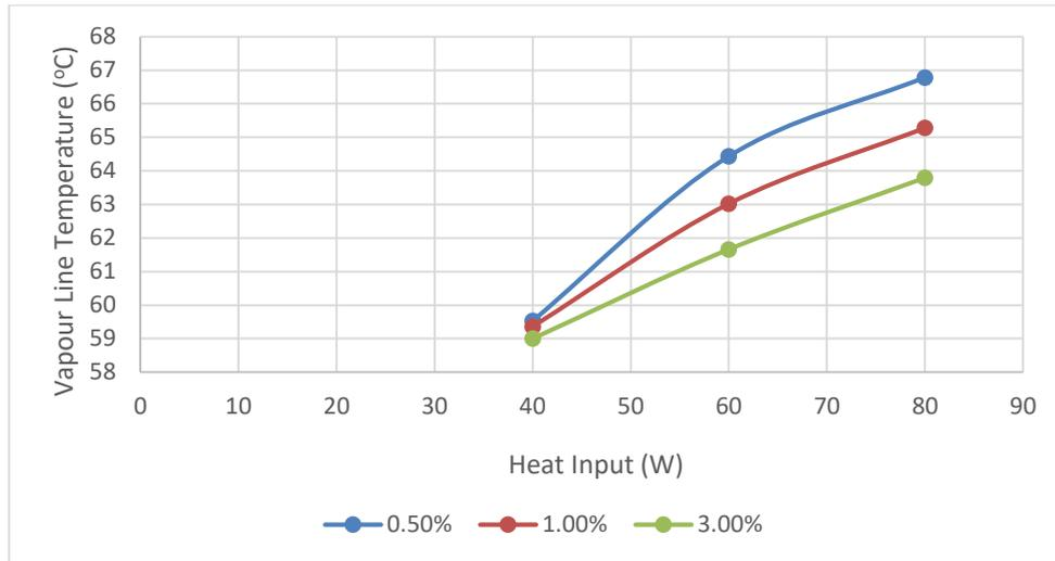
**Fig. 5.** Vapour line temperature versus heat input using various mass concentrations of diamond nanofluid
