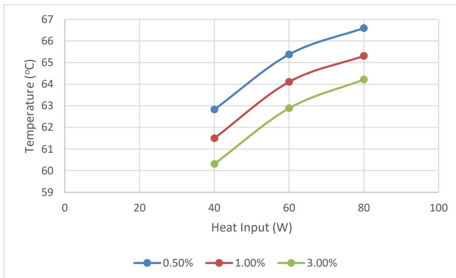
**Fig. 6.** Vapour line temperature versus heat input using various mass concentrations of aluminium nanofluid
