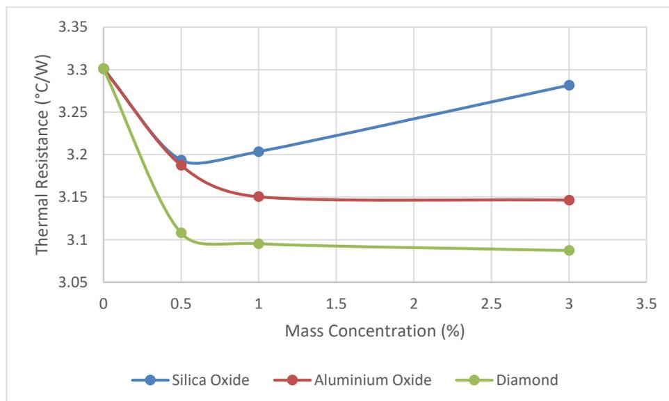
**Fig. 3.** Mass concentration versus thermal resistance with different nanofluids.
