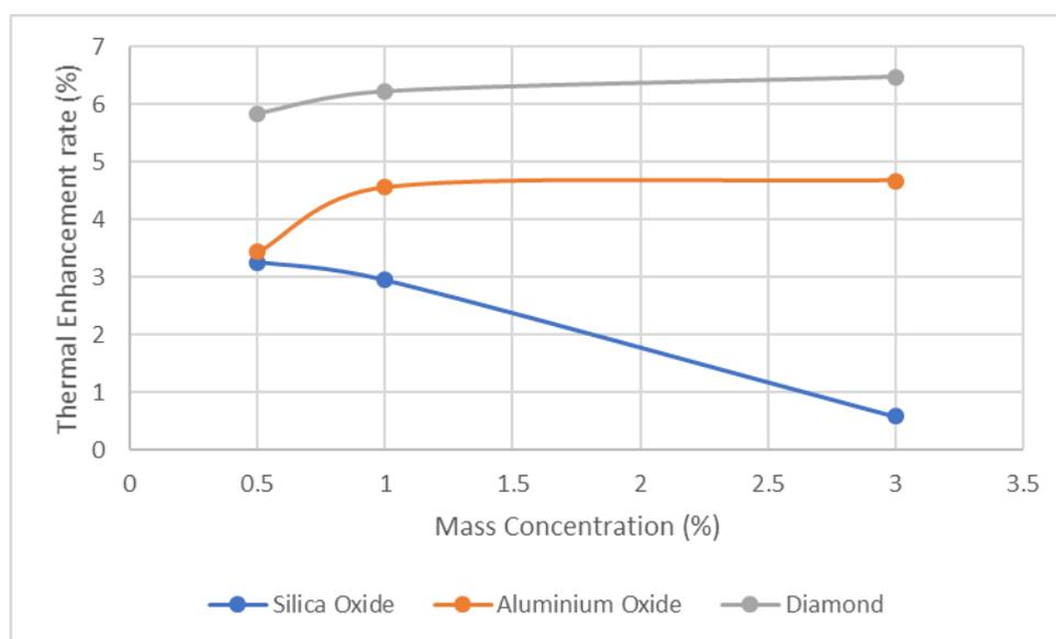
**Fig. 4.** Mass concentration versus thermal enhancement rate with different nanofluids.
