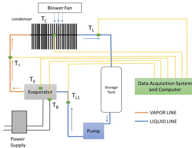
**Fig. 1.** Schematic diagram of experimental rig setup of LHP.
