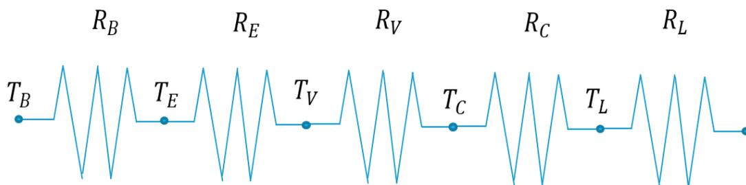
Fig. 2. Thermal resistance network of LHP.
