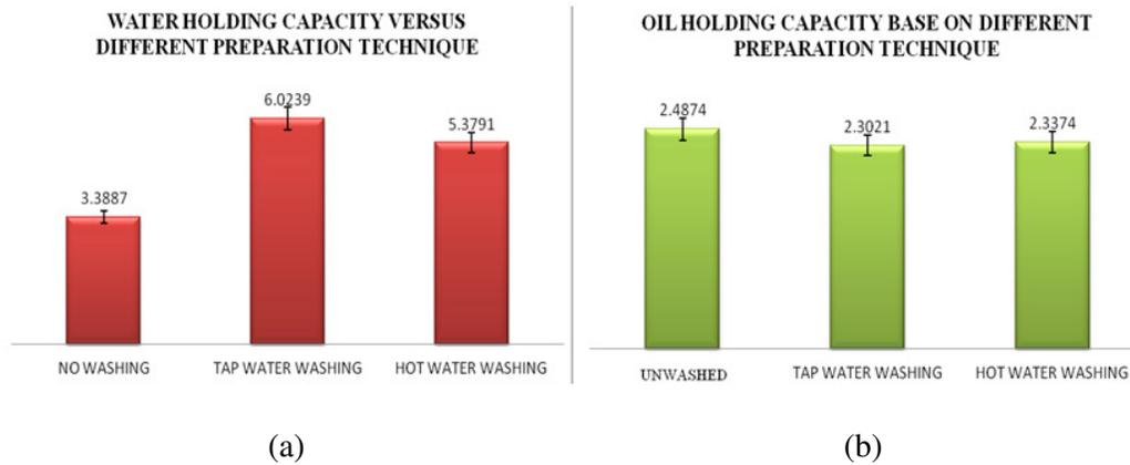
**Figure 1:** (a) Water holding capacity (g water/ g dry weight) and (b) Oil holding capacity (g oil/ g dry weight) of different preparation technique
