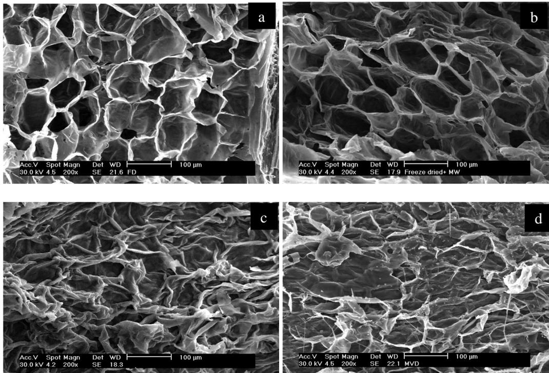
**Figure 4:** Scanning electron micrographs of pineapple core fibers using different drying methods a) freeze dry, FD; b) microwave combined with freeze dry, MFD; c) vacuum dry, VD; d) microwave vacuum dried, MVD
