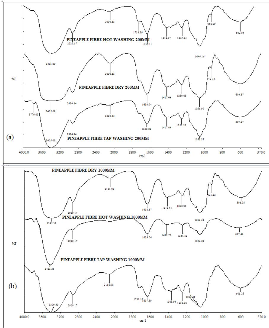
**Figure 3:** Fourier transform infrared (FT-IR) spectroscopy analysis within the range of 4000 to 370  $\text{cm}^{-1}$  for tap, hot water washing and unwashed (control) fiber with particles sizes of a) 200 and b) 1000 micrometres.
