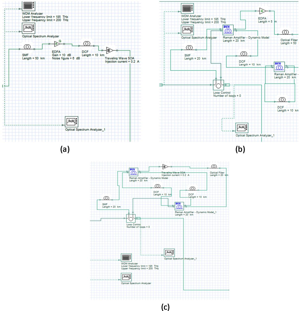
**Fig. 1.** Layout of fiber optical link of DWDM system for various hybrid configurations of optical amplifier (a) Hybrid EDFA-SOA (b) Hybrid EDFA-RAMAN (c) Hybrid RAMAN-SOA
