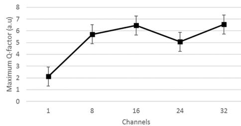
**Fig. 2.** Maximum Q-factor values of DWDM using hybrid EDFA-SOA with injection current 0.2 A
