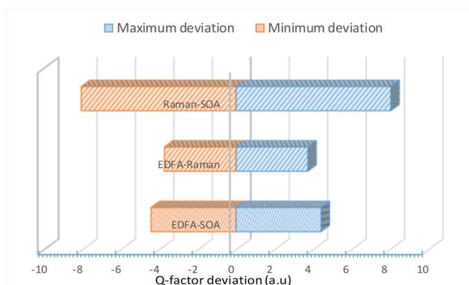
**Fig. 12.** Analyses on received signal's stability at selected channels (1, 8, 16, 24 and 32) between EDFA-SOA, EDFA Raman and Raman-SOA
