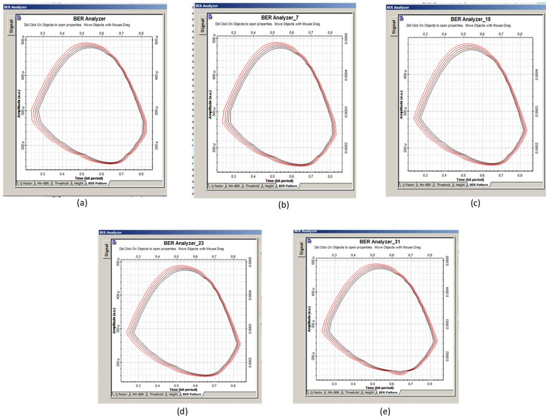
**Fig. 9.** BER pattern for 32 channels DWDM using hybrid RAMAN-SOA Maximum Q-factor for various channels of DWDM using hybrid RAMAN-SOA (a) Channel 1, (b) Channel 8, (c) Channel 16, (d) Channel 24 and (e) Channel 32
