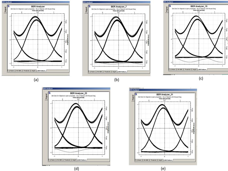
**Fig. 10.** Eye diagram for various channels of DWDM using hybrid Raman-SOA (a) Channel 1, (b) Channel 8, (c) Channel 16, (d) Channel 24 and (e) Channel 32
