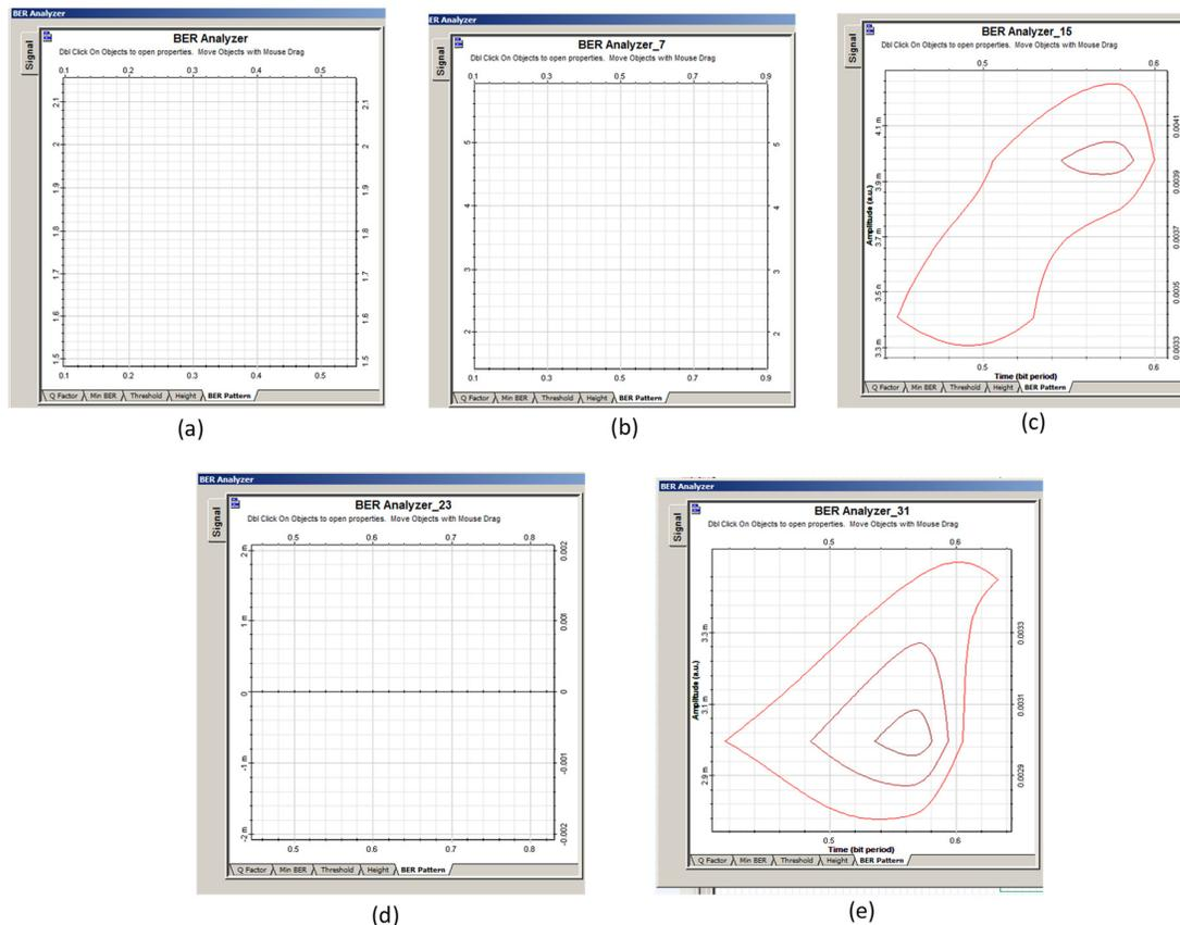
**Fig. 3.** BER pattern various number of channels of DWDM using hybrid EDFA-SOA (a) 1 (b) 8 (c) 16 (d) 24 (e) 32
