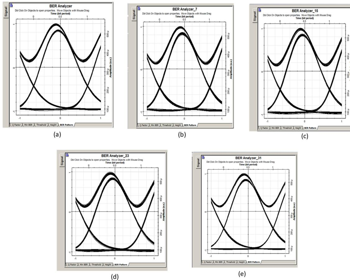
**Fig. 7.** Eye diagram for various channels of DWDM using hybrid EDFA-RAMAN (a) Channel 1, (b) Channel 8, (c) Channel 16, (d) Channel 24 and (e) Channel 32
