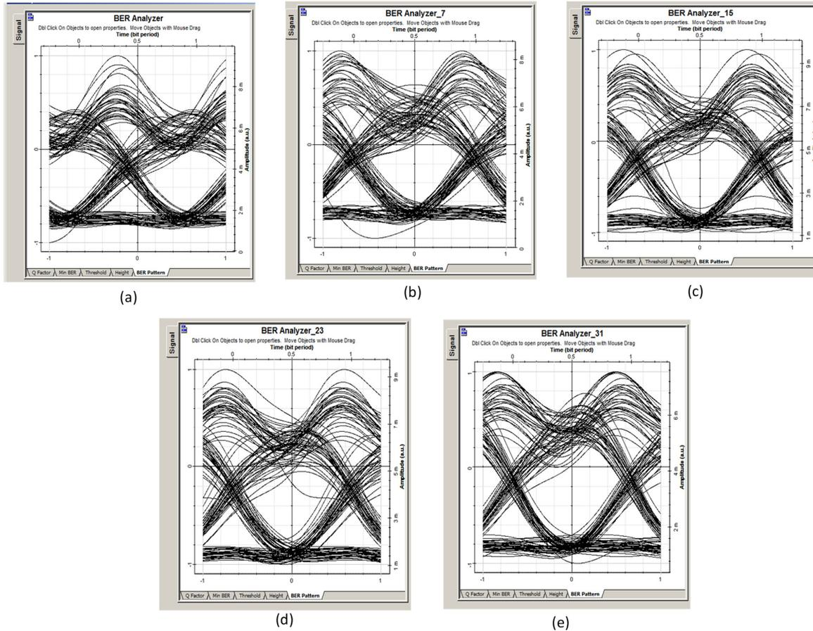
**Fig. 4.** Eye diagram for various number of channels DWDM using hybrid EDFA-SOA (a) 1, (b)8 (c) 16 (d) 24 (e) 32
