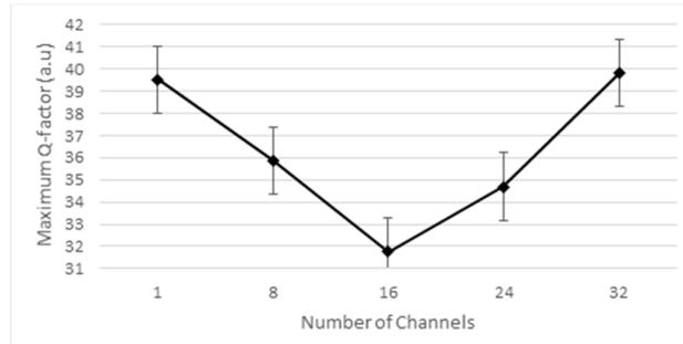
**Fig. 8.** Relationship between maximum Q-factor and various channels of DWDM using hybrid RAMAN-SOA (a) Channel 1, (b) Channel 8, (c) Channel 16, (d) Channel 24 (e) Channel 32
