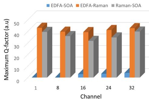
**Fig. 11.** Relationship between maximum Q-factor (a.u) and number of channels for hybrid EDFA-SOA, EDFA-RAMAN and RAMAN-SOA
