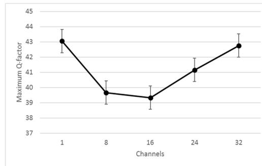
**Fig. 5.** Maximum Q-factor for various channels of DWDM using hybrid EDFA-RAMAN
