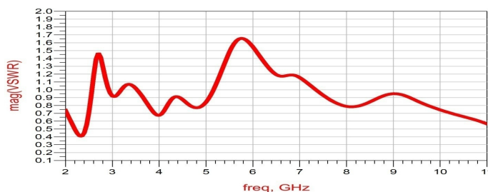
Fig. 6. Simulated VSWR of the proposed design
