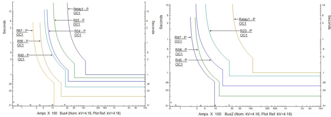
Fig. 5. CCT of forward relays for case 1 and case 9 respectively
