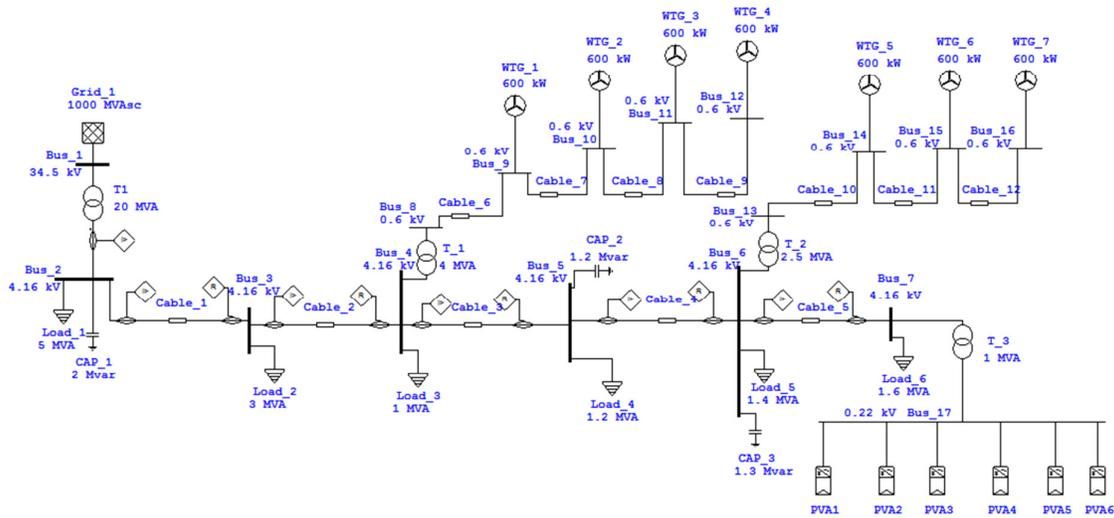
**Fig. 2.** Details of the tested system in ETAP
