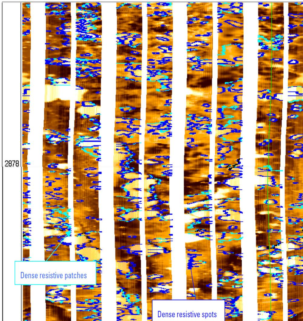
**Figure 3:** FMI calibrated images highlighting resistive features / areas in a carbonate section. Contoured in blue are resistive or dense features; patches are in cyan while spots are in blue. The spots are dense or resistive features / areas where dimensions are less than  $0.003\text{m}^2$
