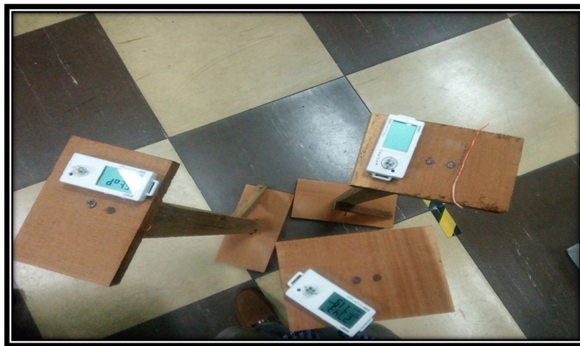
Fig. 5. A View of the Hobo Weather Data Loggers (HWDL)
