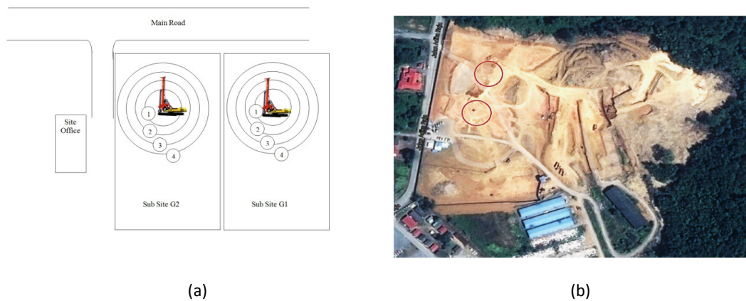
Fig. 1. (a) Schematic diagram and (b) site layout for location of both piling machines in Pengkalan Hulu Perak
