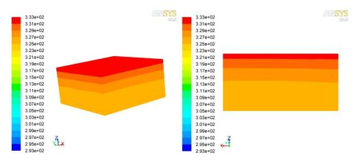
Figure 6: Contour view of asphalt pavement without water circulation
