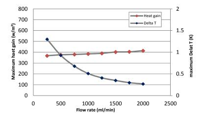
Figure 11: Comparison between the maximum heat gain with different volume flow rates of the current study for validation purpose
