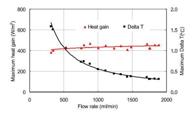
Figure 10: Comparison between the maximum heat gain with different volume flow rates based on Shaopeng's study [5]
