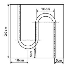
Figure 1a: Schematic diagrams of geometry Fluent
