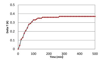
Figure 9: Temperature between inlet and outlet water with varying time of the current study for validation purpose
