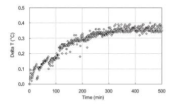
Figure 8: Temperature between inlet and outlet water with varying time based on Shaopeng's study [5]
