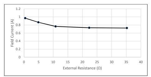
Fig. 10. Effects of external resistance addition towards the motor's field current
