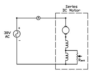
Fig. 9. Experimental setup of field resistance control method
