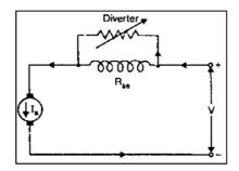
Fig. 4. Field diverter method
