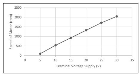
Fig. 15. Effects of the separate variable voltage supply towards the motor's speed
