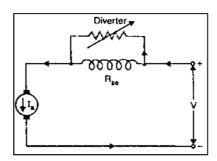
Fig. 3. Field diverter method
