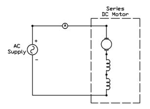
Fig. 14. Experimental setup of terminal voltage control method
