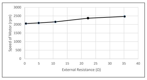
Fig. 11. Effects of external resistance addition towards the speed of series DC motor
