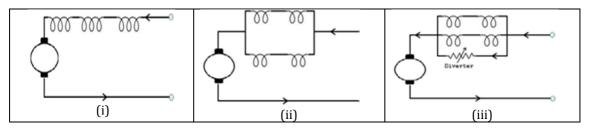
Fig. 7. Paralleling field coils
