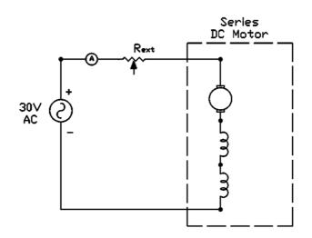
Fig. 12. Experimental setup of armature resistance control method
