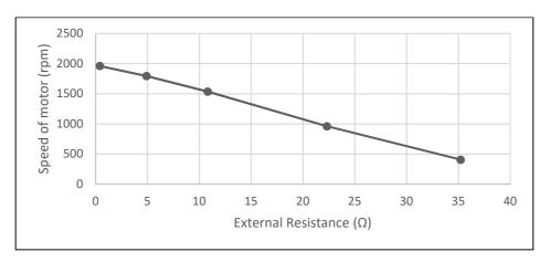
Fig. 13. Effects of external resistance in series with the motor towards the motor's speed
