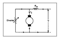
Fig. 5. Armature diverter method
