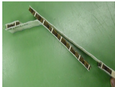
Fig. 4. Peel condition of SN 1 after conducted vertical 90° test
