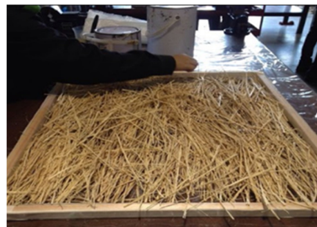
Figure 3b: Bamboo fiber arrangement in multidirection before resin pouring.
