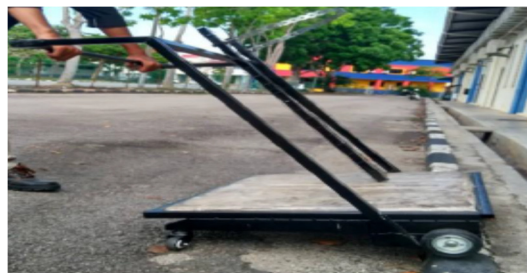
Figure 7: Fabricated welding cart with bamboo composite base
