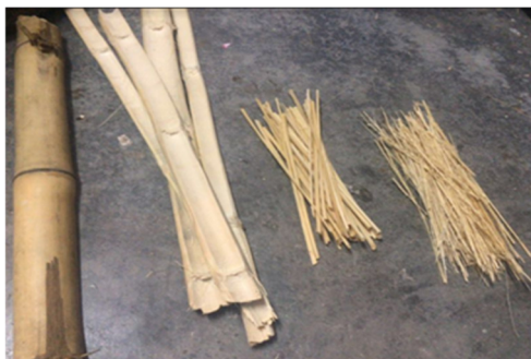
Figure 3a: Bamboo fiber extraction from raw material.
