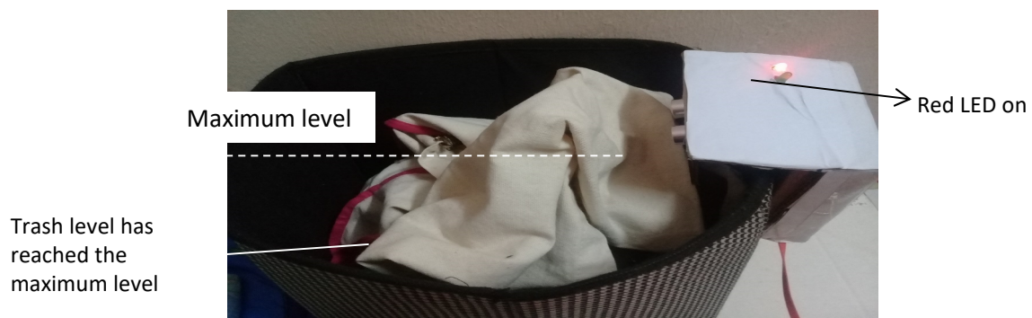
Fig. 5. High condition of trash level
