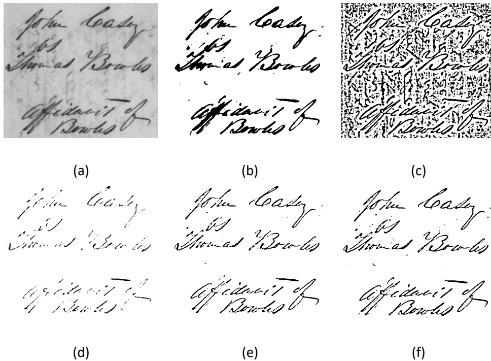
Fig. 2. Comparison of resulting images; (a) original, (b) Otsu method, (c) Niblack method, (d) Bernsen method, (e) Nick method, and (f) Proposed method
