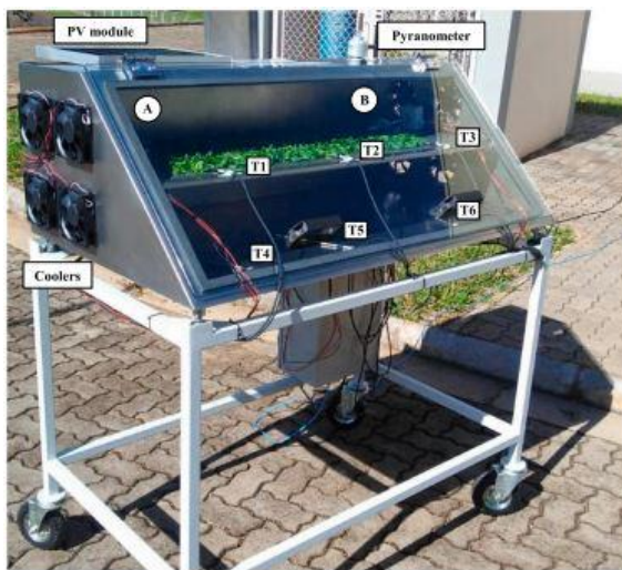
Fig. 7. Direct solar dryer [24].
