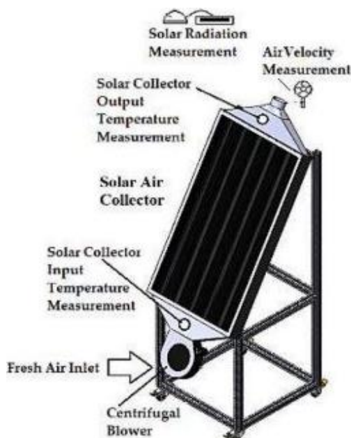
Fig. 1. Experimental setup and measurement points [2]. Fig. 2. Front view of a flat solar collector [4].
