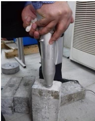
**Fig. 11.** Rebound hammer test
