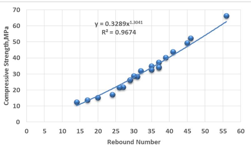
**Fig. 12.** Compressive strength vs rebound number
