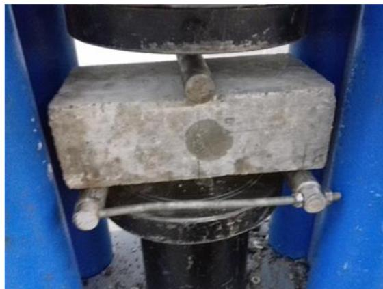
**Fig. 8.** Flexural strength test procedure
