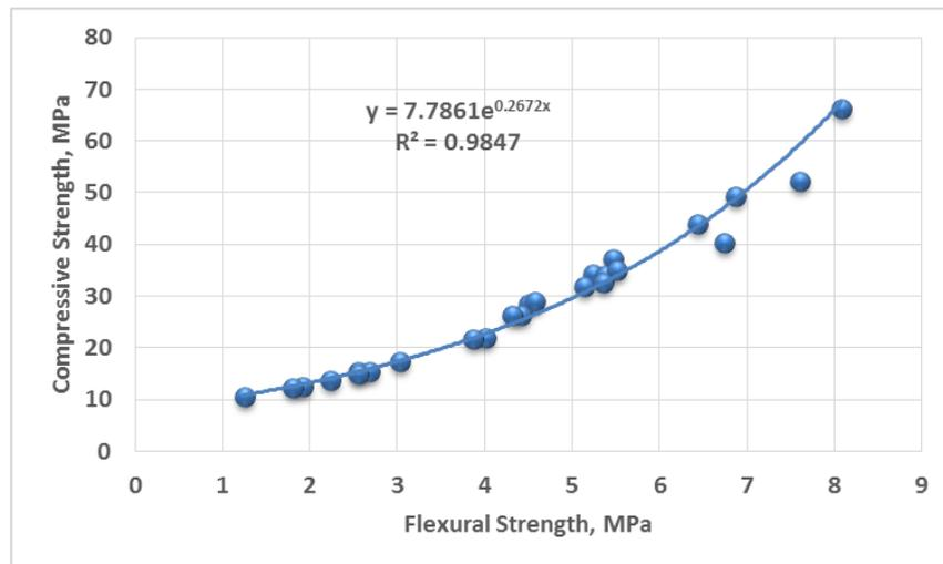
**Fig. 9.** Compressive strength vs flexural strength of geopolymer concrete bricks
