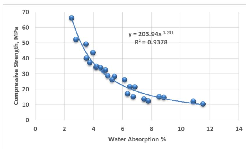
**Fig.3.** Compressive strength vs water absorption % of geopolymer concrete bricks.
