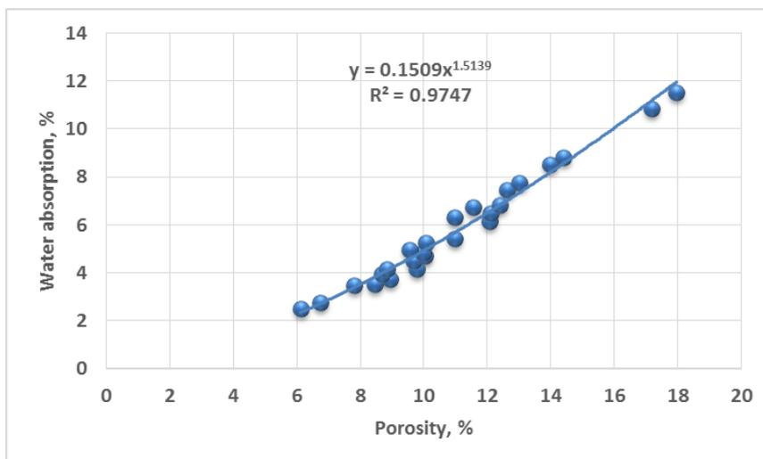
Fig. 5. Relationship between water absorption and apparent porosity of geopolymer concrete bricks
