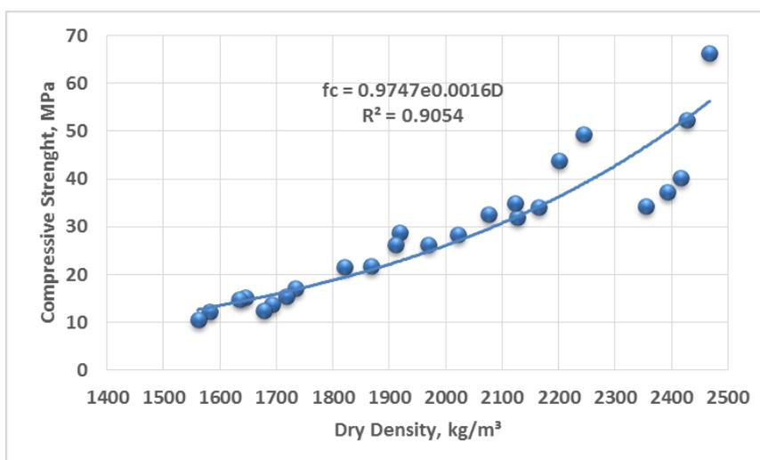
**Fig.7.** Compressive strength vs dry density of geopolymer concrete bricks
