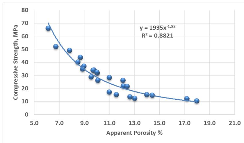
**Fig. 4.** Compressive strength vs apparent porosity % of geopolymer concrete bricks
