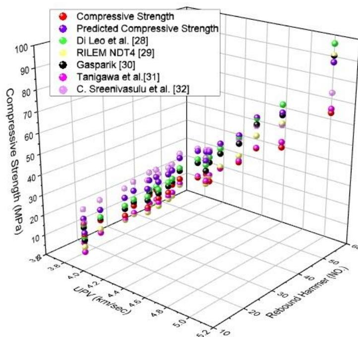
**Fig. 14.** Comparing the experimental compressive strength with proposed equation and various References equations.
