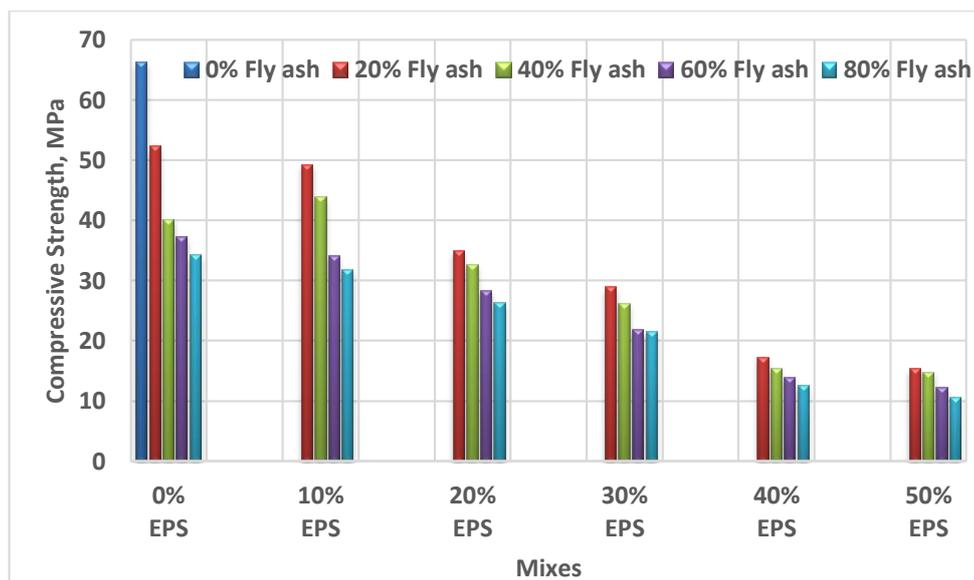
Fig. 15. Effect of EPS and fly ash % on compressive strength of geopolymer concrete bricks
