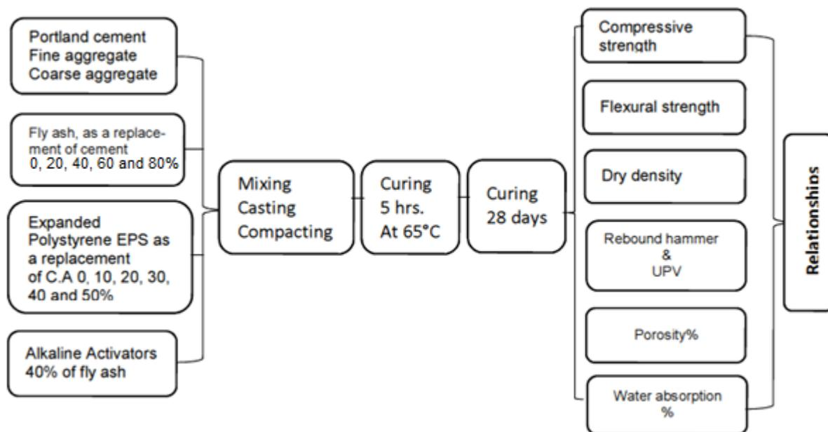
Fig. 1. Methodology of the experimental program
