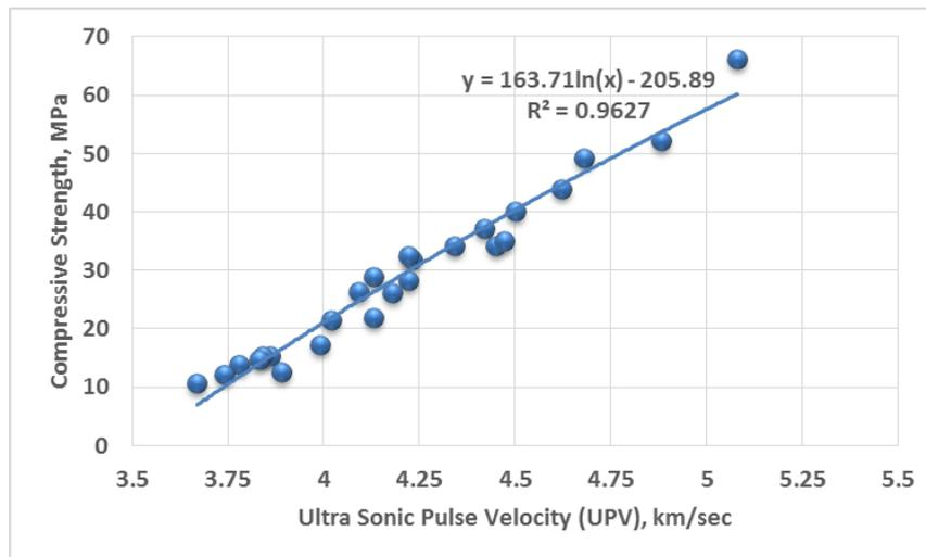
**Fig. 13.** Compressive strength vs UPV of geopolymer concrete bricks
