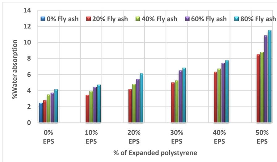
**Fig. 2.** water absorption% vs expanded polystyrene% of geopolymer concrete bricks
