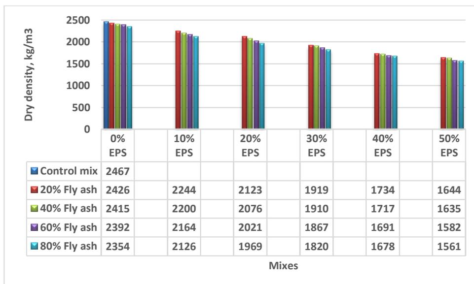
**Fig. 6.** Dry density of different geopolymer concrete mixes
