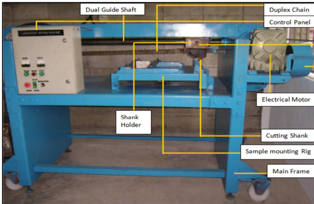
Fig. 4. Laboratory ripping test
