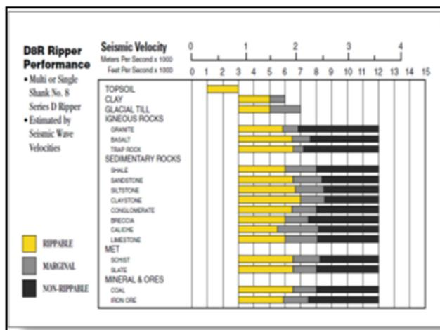
Fig. 2. Chart of ripper performance for D8 [9]
