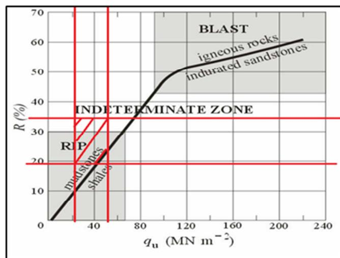
Fig. 1. Rebound number (R) plotted unconfined compression strength (qu) [4]
