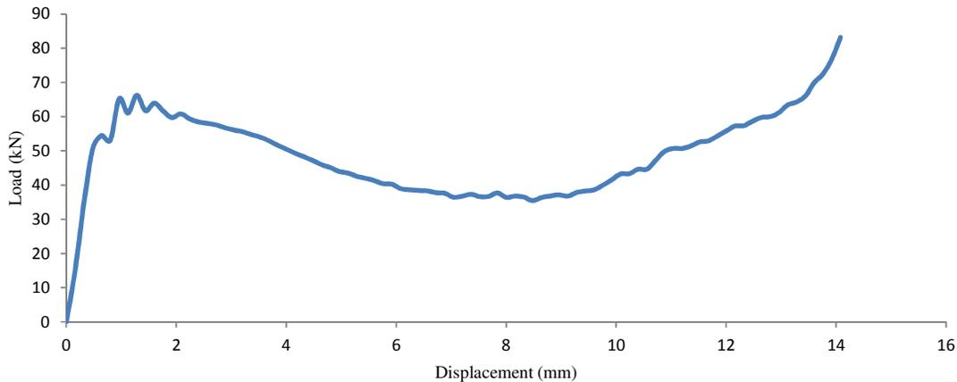
**Fig. 7.** Load-displacement curve for core cell size 20x20 mm
