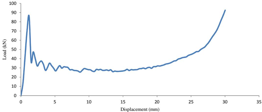
**Fig. 10.** Load-displacement curve for core cell size of 30x40 mm
