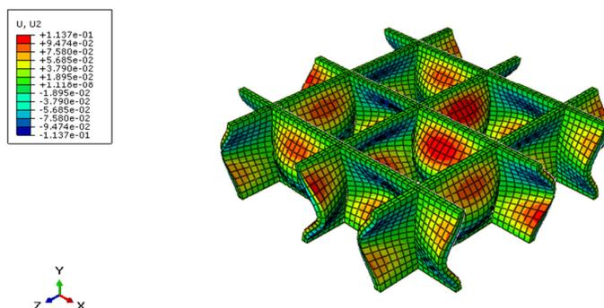
Fig. 6. the initial imperfection behavior of the model with size of 20x20 mm
