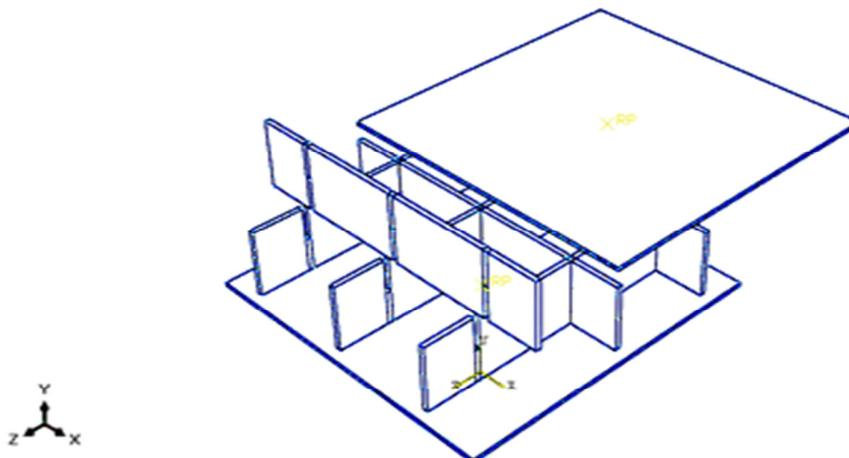
**Fig. 2.** The assembly of interlocking core with upper and bottom platens
