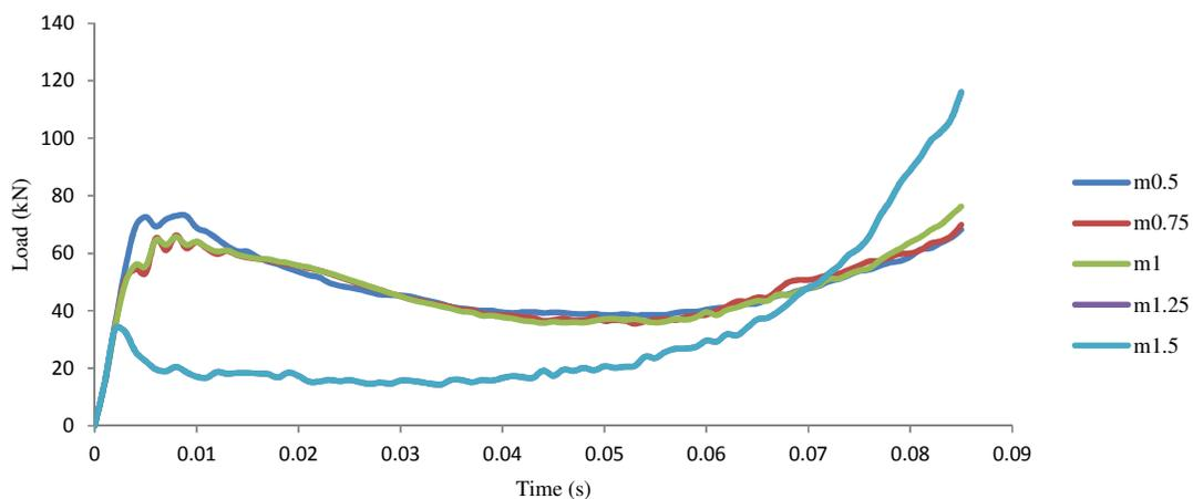
Fig. 3. Effect of changing meshing size on the reaction force
