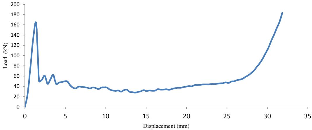
**Fig. 12.** Load-displacement curve for core cell size 50x40 mm
