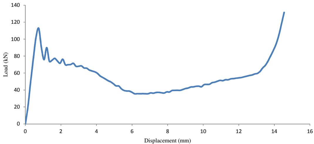
**Fig. 9.** Load-displacement curve for core cell size 30x20 mm
