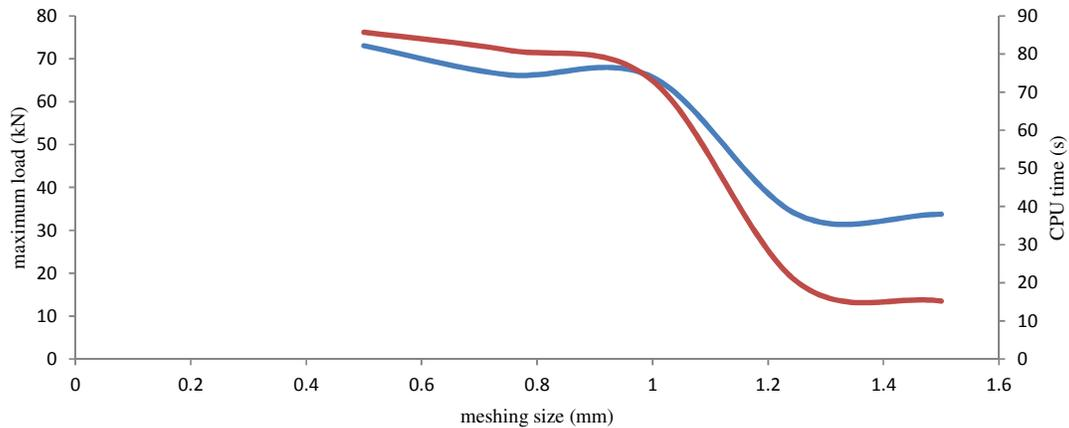
**Fig. 4.** Relationship between meshing size and both max load and CPU time
