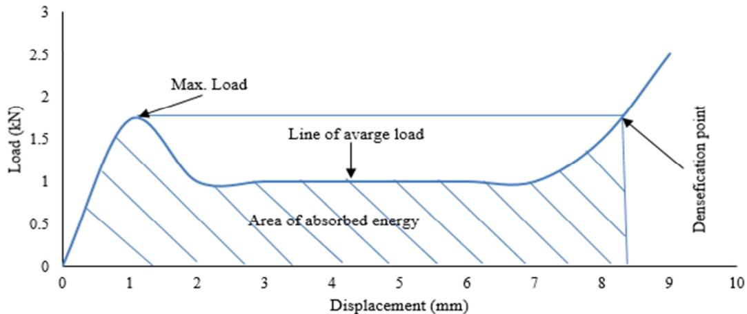
**Fig. 5.** Shows the area of absorbed energy in load-displacement curve [27]
