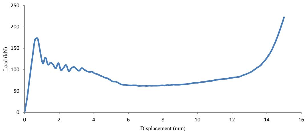
**Fig. 11.** Load-displacement curve for core cell size 50x20 mm
