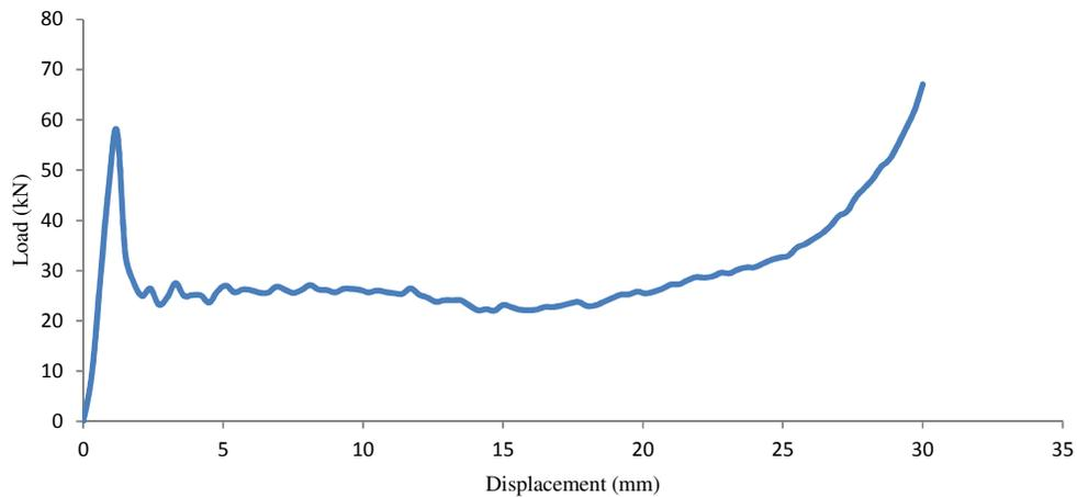
**Fig. 8.** Load-displacement curve for core cell size 20x40 mm
