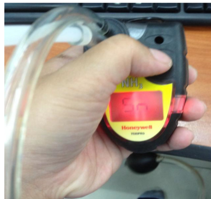
Figure 3: Setting-Up The ToxiPro ( \text{NH}_3 Gas Detector)
