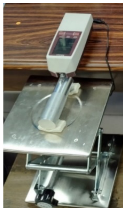
Fig. 2. The Measurement Process of Surface Roughness
