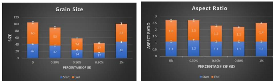
**Fig. 2.** a) Grain size of silicone. b) Aspect ratio of silicone particles as a result of Gd addition.
