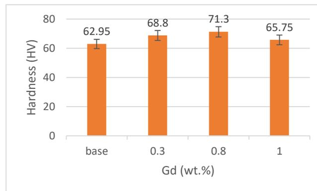
**Fig. 8.** Hardness test results for base alloys with various amounts of Gd modifications.
