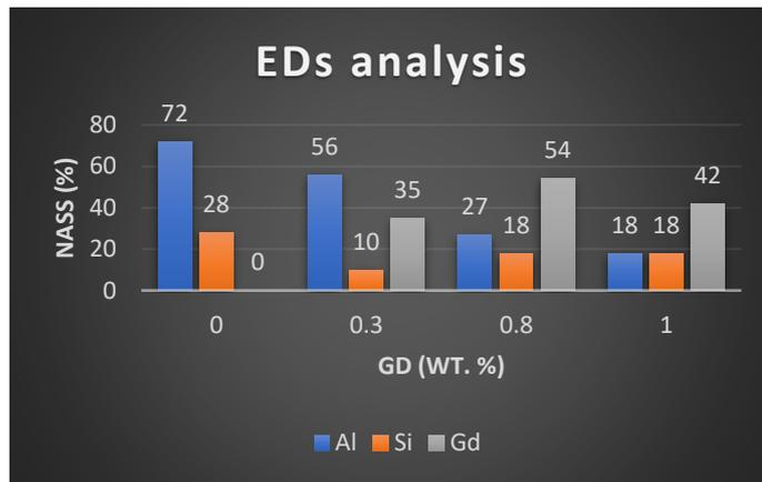
**Fig. 5.** The EDS analysis of Al-18Si alloy with Gd wt. %
