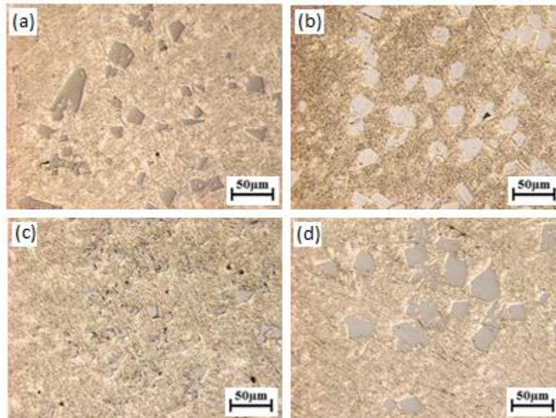
**Fig. 1.** Optical images of Al-18Si with Gd addition, (a) 0, (b) 0.3, (c) 0.8 and (d) 1.0 wt.% need to insert the optical images
