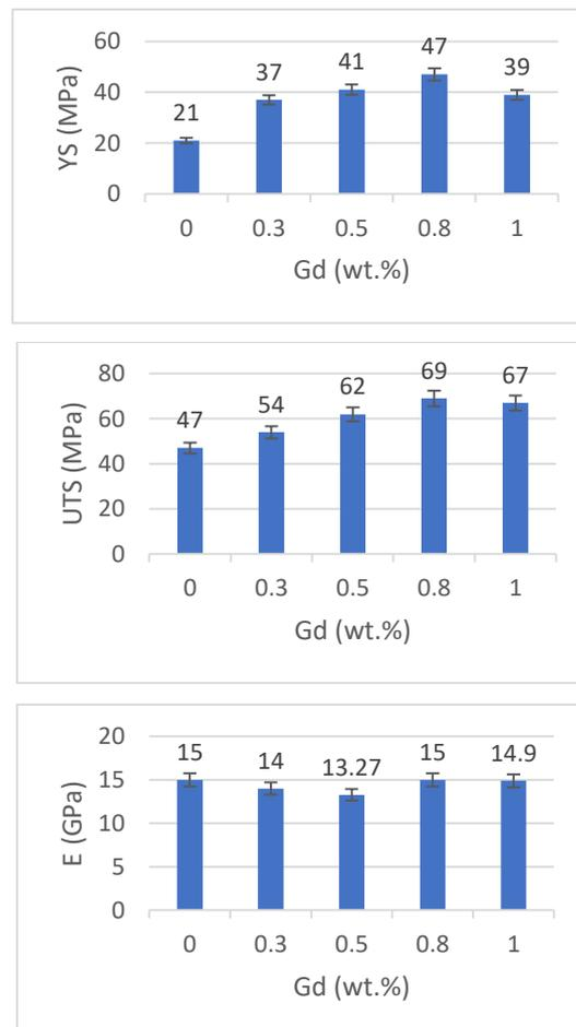
**Fig. 7.** Tensile test results for base alloys with various amounts of Gd modifications, including YS, UTS, and E.
