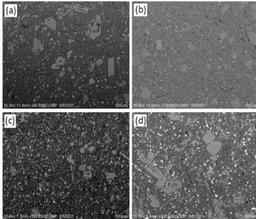
Fig.3 SEM images of Al-18Si with Gd addition, (a) 0, (b) 0.3, (c) 0.8 and (d) 1.0 wt.%
