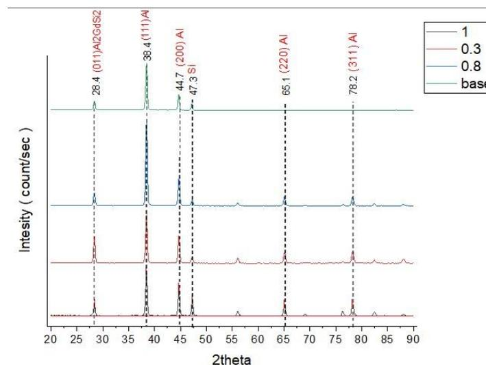
**Fig. 6.** Various amounts of Gd additions produce different X-ray diffraction patterns
