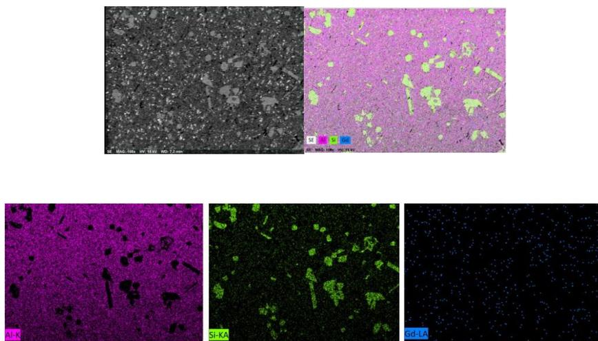
Fig. 4. Elemental dot mapping of modified sample containing 0.8 wt.% Gd
