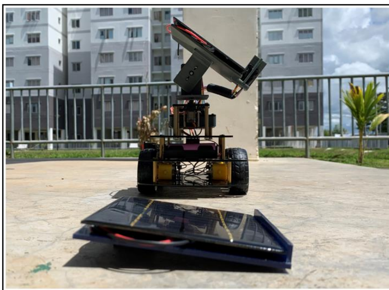
Fig. 10. Fixed solar panel slanted at 7°
