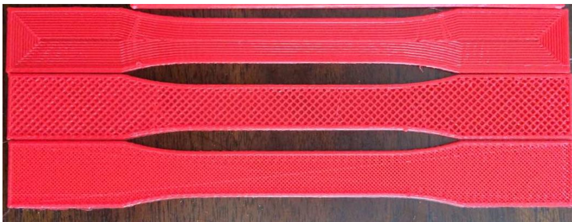
Fig. 7. From above, concentric line, line, and grid pattern
