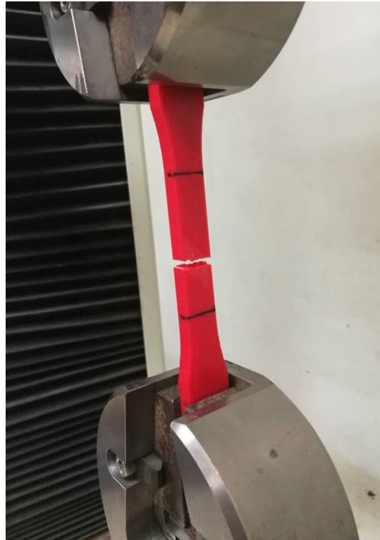
Fig. 9. Sample PLA fabrication undergoing tensile test
