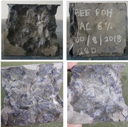
Fig. 5. Unsatisfactory Failure of Specimen Concrete with 6% of Clam Shell Ash as Replacement of OPC
