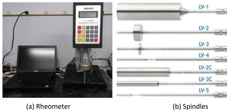
Fig. 7. The rheometer and the spindles used in this investigation (the LV-5 spindle was selected after preliminary trials)
