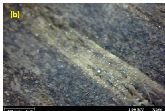
Fig. 2. Microscopic images from the surface of OPS aggregates (a) heat treatment and (b) without heat treatment
