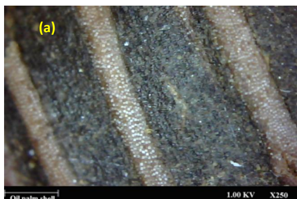
Fig. 2. Microscopic images from the surface of OPS aggregates (a) heat treatment and (b) without heat treatment
