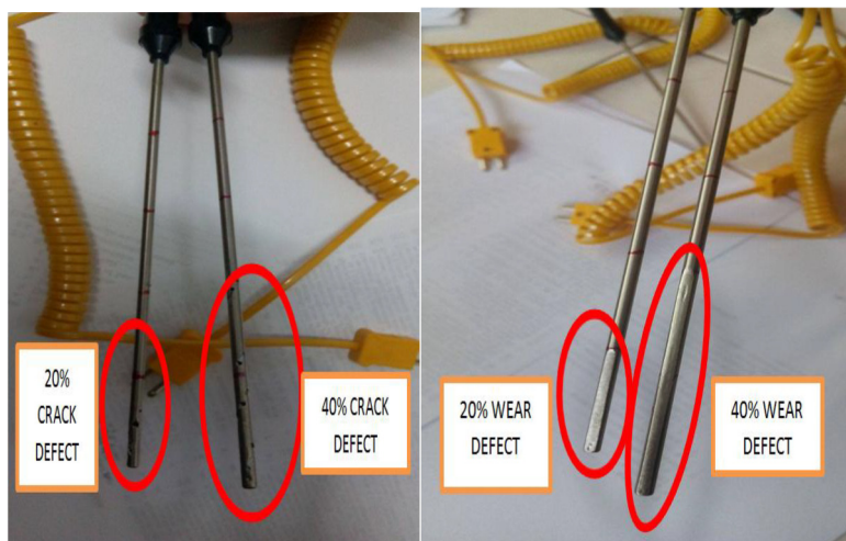
Fig. 1. Defects on the Thermocouple Sample
