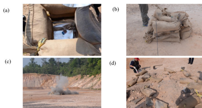
Fig. 2. Photographs showing (a) Arrangement of home-made bomb surrounded by sandbags, (b) Sandbag used to cover the bomb from above, (c) Scene immediately after the explosion, and (d) Debris from the seat of explosion ready for collection
