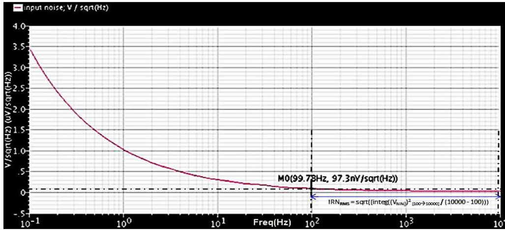
Figure 12: Total Simulated IRN of I/Q Baseband Amplifier & Filter
