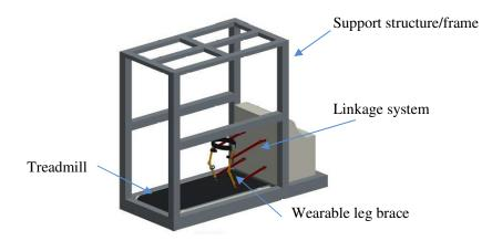
Figure 2: 3D model of the design
