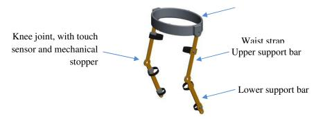
Figure 4: The wearable leg brace
