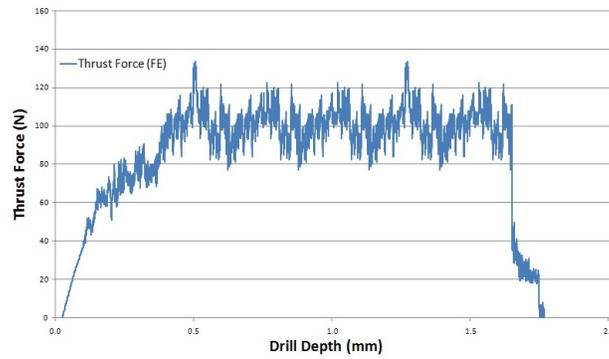
**Figure 3(b):** Simulation result of thrust force
