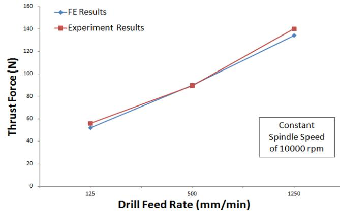
**Figure 5(a):** Thrust force analysis (Experiment and FE)
