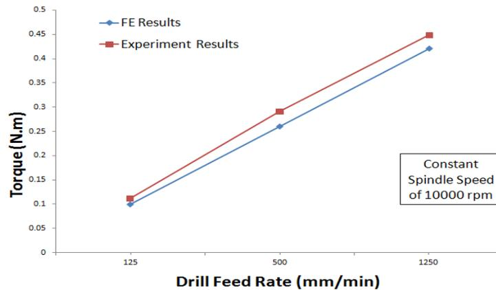
**Figure 5(b):** Torque analysis (Experiment and FE)
