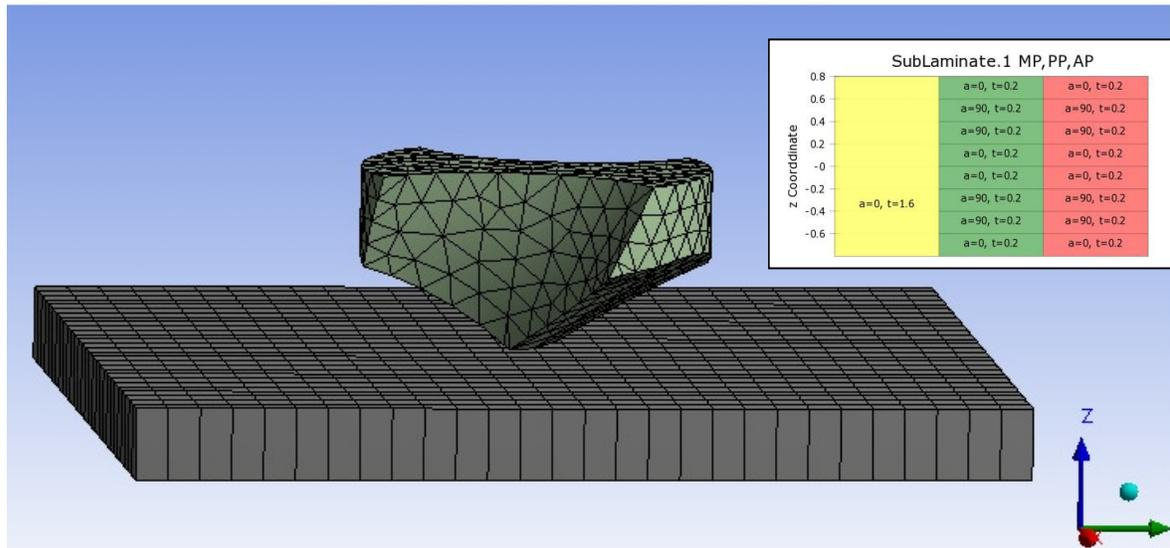
**Figure 2:** Finite element model of VTM264 CFRP Laminate &PCD twist drill
