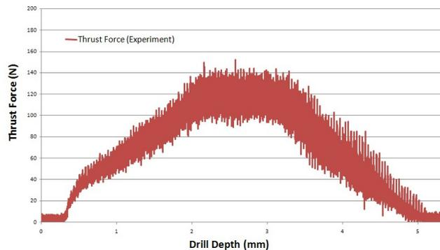
**Figure 3(a):** Experimental result of thrust force
