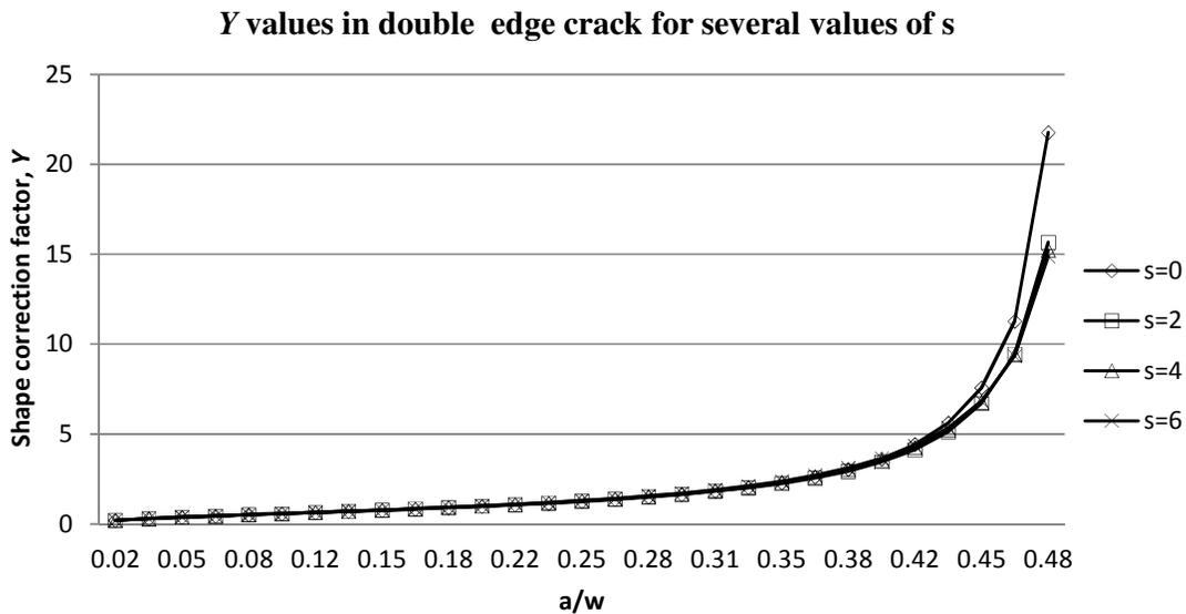
**Figure 4:** Graph of Y values in double edge crack for several values of crack distance, s
