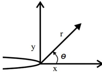
**Figure 2:** Crack tip coordinates [5]
