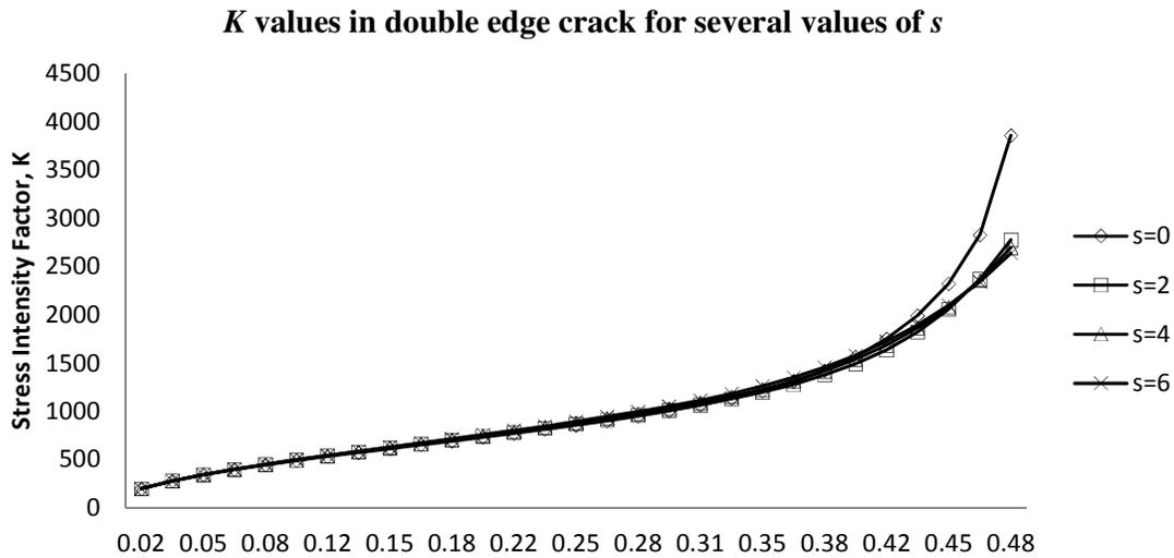
**Figure 3:** Graph of K values in double edge crack for several values of crack distance, s
