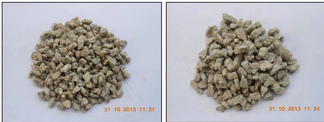
Figure 1: (a) 5 to 8 mm size of aggregate, and (b) 8 to 10 mm size of aggregate.
