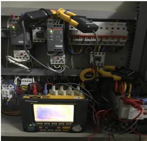
Fig. 2. (a) Power analyzer to measure compressor power
